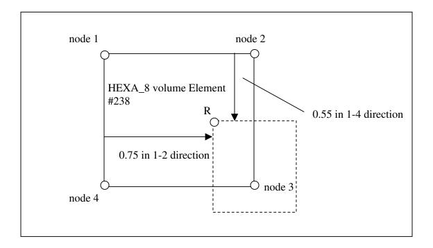
The HEXA\_8 volume element has been appropriately numbered, using information given in "Unstructured Grid Element Numbering Conventions." In this example, it is the 1-2-3-4 face of the volumetric element that is abutting with the other zone (but it could be any of its 6 faces).
