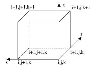
For unstructured grids, InterpolantsDonor is defined only for the basic linear element types: BAR\_2, TRI\_3, QUAD\_4, TETRA\_4, PYRA\_5, PENTA\_6, and HEXA\_8.
