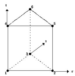
$$\begin{aligned} W_1 &= (1 - r - s)(1 - t) \\ W_2 &= r(1 - t) \\ W_3 &= s(1 - t) \\ W_4 &= (1 - r - s)t \\ W_5 &= rt \end{aligned}$$
